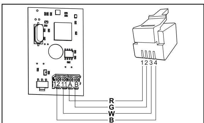
Fig 18: Connecting the humidity- and temperature sensor - Combi Elite
