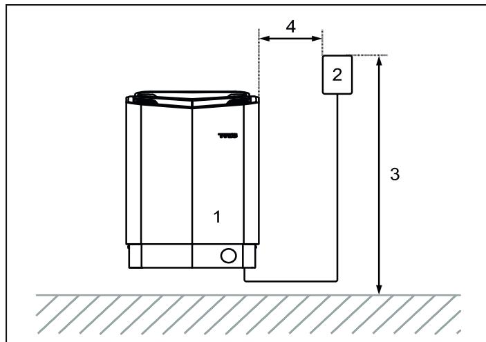
Figure 6: Safety distance / installation height, control panel
